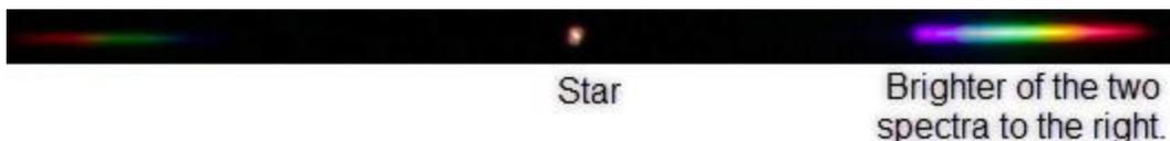
To confirm and fine-tune the Star Analyser's rotational position, capture an image using any imaging software you wish. If the spectrum does not appear to be horizontal, rotate the grating a bit and capture another test image. Don't worry if this fine-tuning takes a few tries. This is a trial-and-error process.
