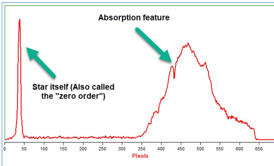
The graph should have dips in it similar to the one at about 425 pixels in the above image. Absorption features are caused, for example, by the star's Hydrogen absorbing specific wavelengths.
