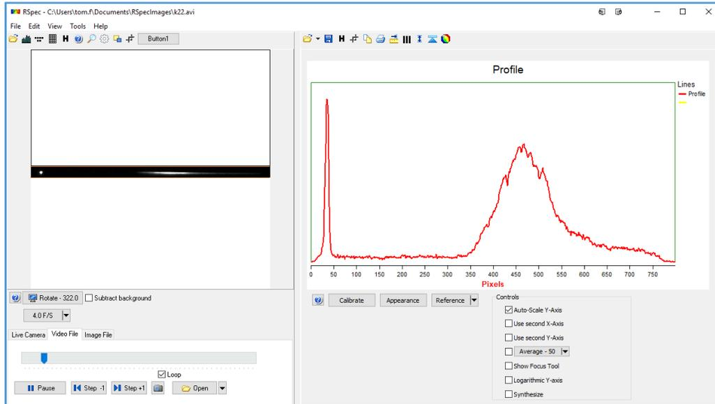
The left panel of this RSpec screen contains the image as seen through the telescope or camera lens; the right panel contains a profile graph that we will discuss in a moment.
