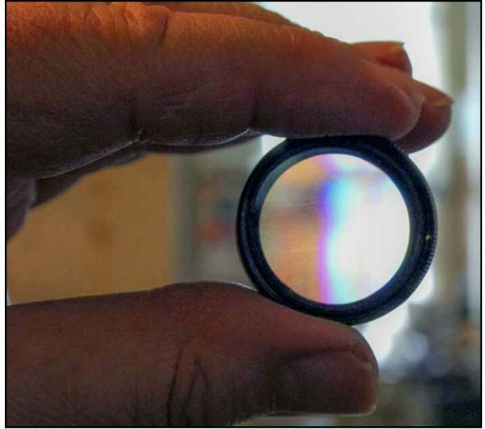
The Star Analyser 100 1.25" filter cell and looking through the cell at the grating and spectra
