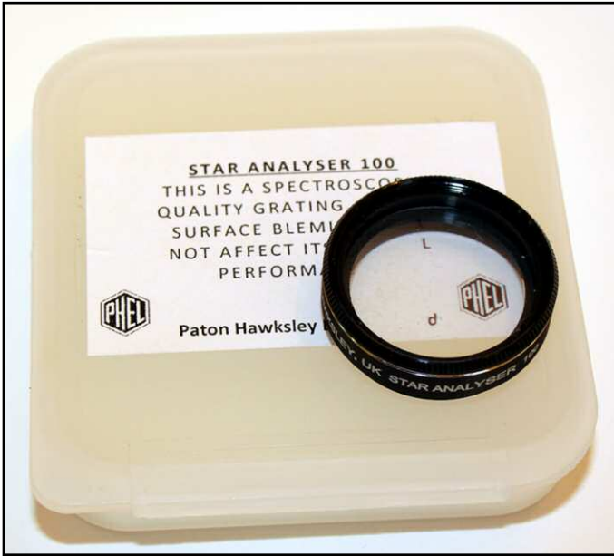
The Star Analyser 100 1.25" filter cell and looking through the cell at the grating and spectra
